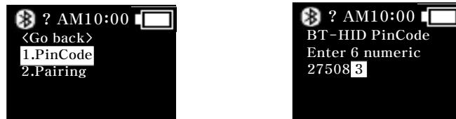
Using up/down button changing the digit and complete with scan button.
