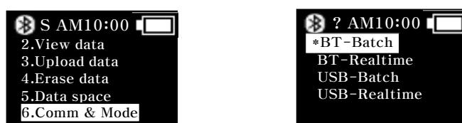
BT-Batch: After storing barcode data, transmit data by “5.Upload data” menu via Bluetooth.
