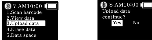
When is ? then, Bluetooth is disconnected. After Bluetooth is connected with S or H, you can transmit data.
