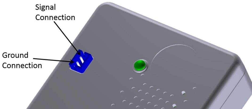
**Figure 2-1: The Smart Room Sensor external connector signals.**
