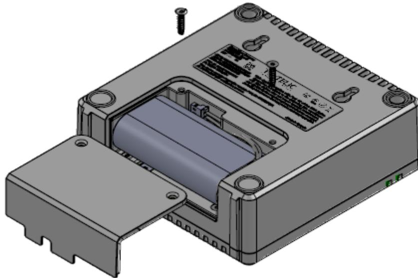
**Figure 6: Battery Installation**
