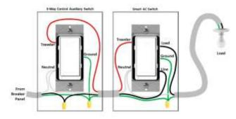
Note: An electrical box ground wire is required.
