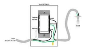
Note: An electrical box ground wire is required.
