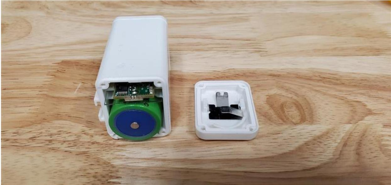
**Figure 2-9: Battery Polarity Markers and Insertion**
