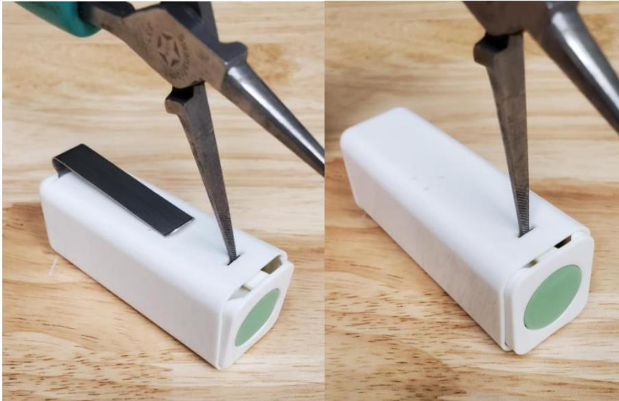
**Figure 2-5: Using a Tool to Release the End-Cap**
