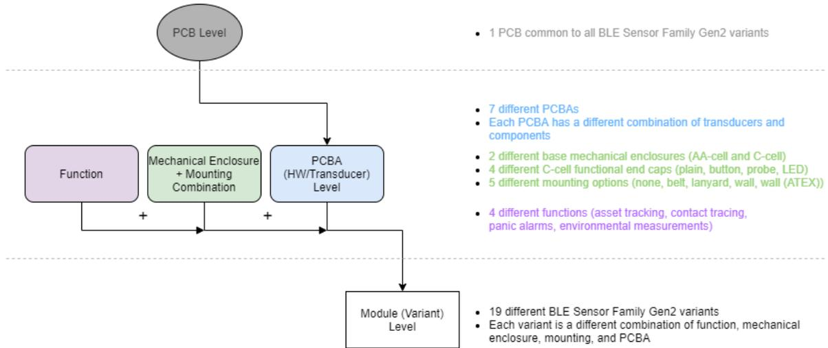
**Figure 1-1: Gen2 BLE Sensor Family Groupings and Hierarchy**
