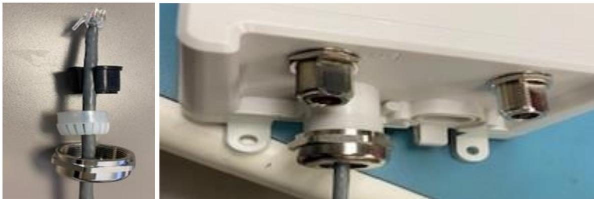
Figure 10: Kona Enterprise Gateway Module Cable Gland
