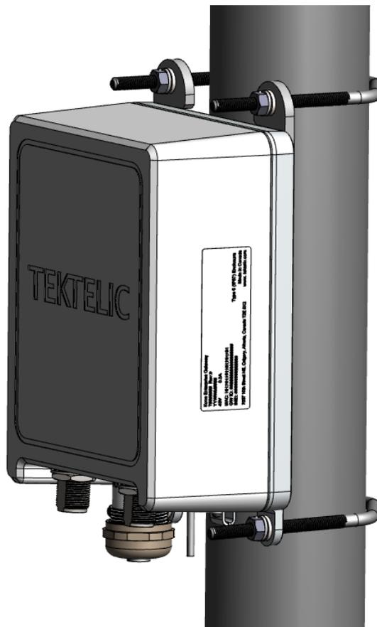
Figure 8: Kona Enterprise Gateway Module Pole Mounting Orientation
