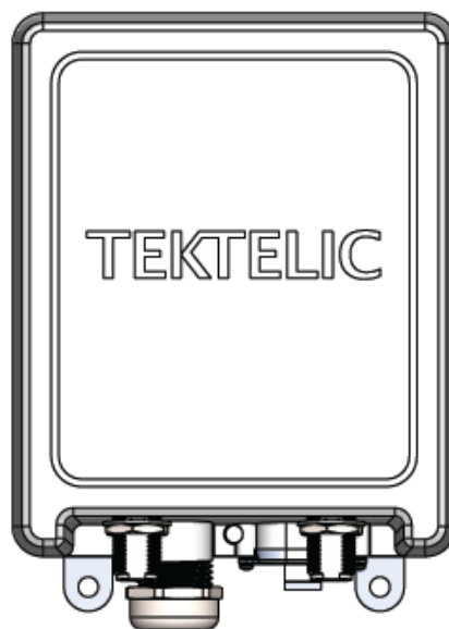
Figure 6: Kona Enterprise Gateway Module Wall Mounting Orientation
