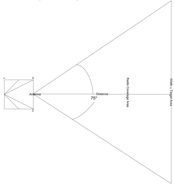
The first step in achieving adequate radio coverage is determining the area where the customer requires increased operations. Once the area has been identified, the distance of the antenna from the target coverage area is calculated as follows:
