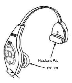
To replace the headband pad, remove the worn/damaged pad by peeling it from the back of the battery housing. Remove protective backing from new pad and press it into place on the back of the battery housing.
