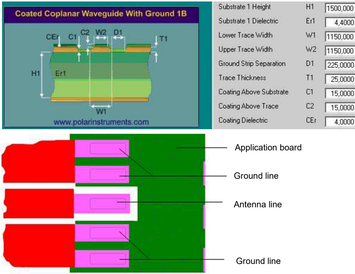
Figure 43: Micro-Stripline on 1.5mm Standard FR4 PCB - example 2
