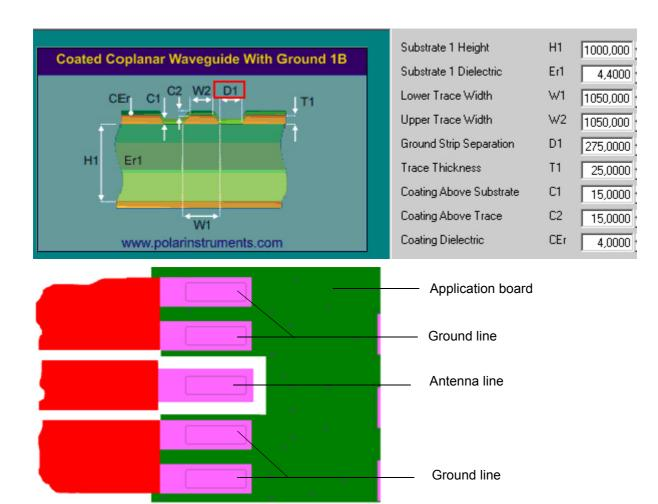
Figure 8: Micro-Stripline on 1.0mm Standard FR4 PCB - example 2
