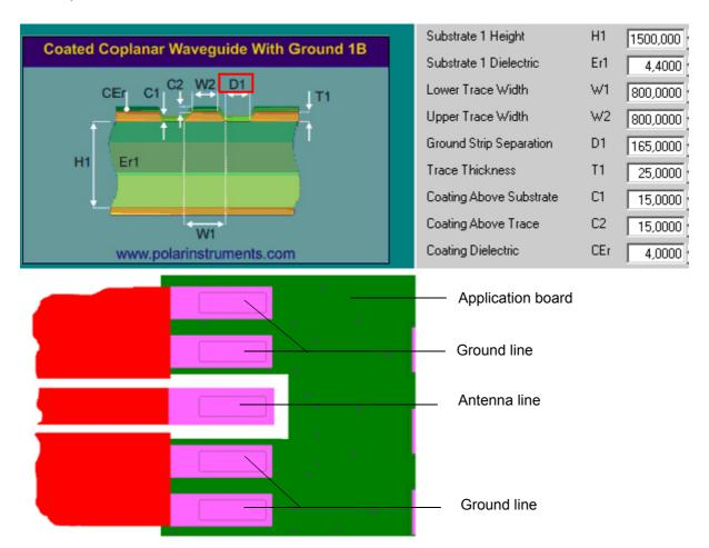
Figure 9: Micro-Stripline on 1.5mm Standard FR4 PCB - example 1
