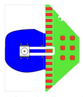
Figure 11: Routing to application's RF connector - top view
