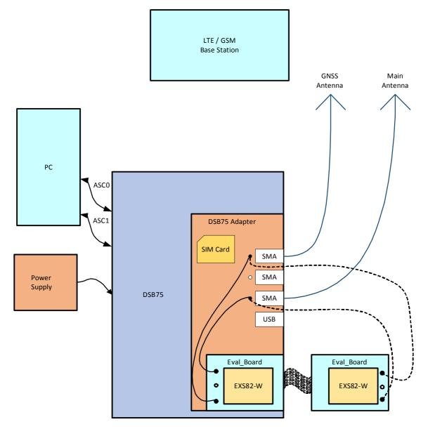
Figure 16: Reference equipment for type approval
