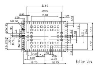
Figure 15: Dimensions of EXS82-W (all dimensions in mm)
