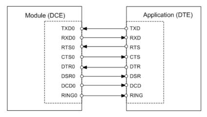
Figure 3: Serial interface ASC0
