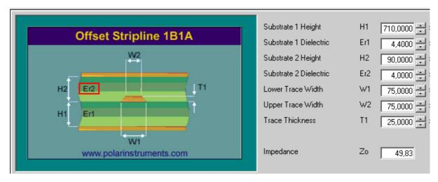
Figure 6: Embedded Stripline with 65µm prepreg (1080) and 710µm core
