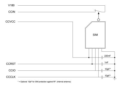
Figure 5: External UICC/SIM/USIM card holder circuit
