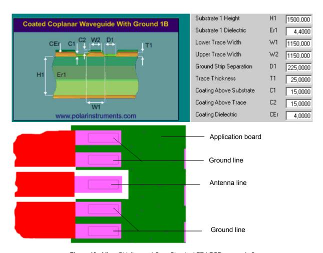
Figure 10: Micro-Stripline on 1.5mm Standard FR4 PCB - example 2
