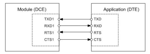
Figure 4: Serial interface ASC1
