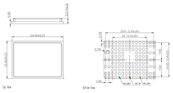
Figure 56: Dimensions of TX82-W, TX62-W-B and TX62-W-C (all dimensions in mm)
