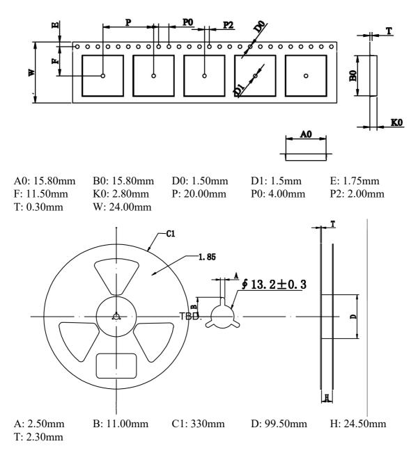
Figure 63: Carrier tape (TX62-W only)
