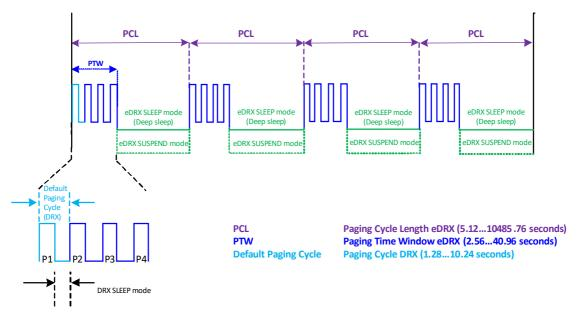
Figure 46: eDRX based paging and power saving in LTE Cat M1 and Cat NB1/2 networks
