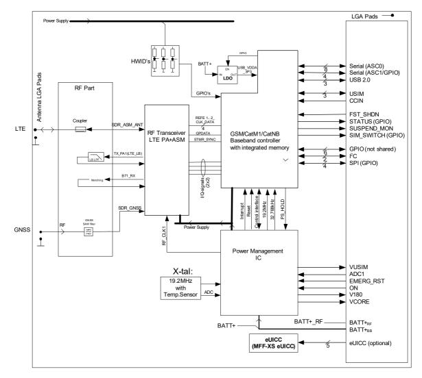
Figure 3: TX62-W block diagram
