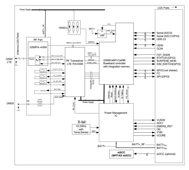
Figure 2: TX82-W block diagram
