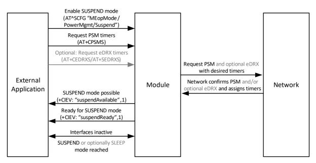
Figure 41: Handshake for entering the module's SUSPEND mode
