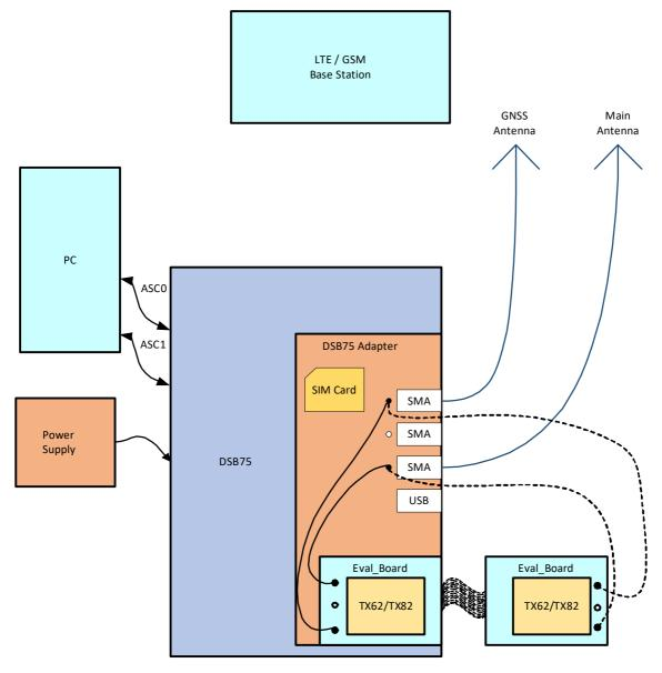
Figure 75: Reference equipment for type approval
