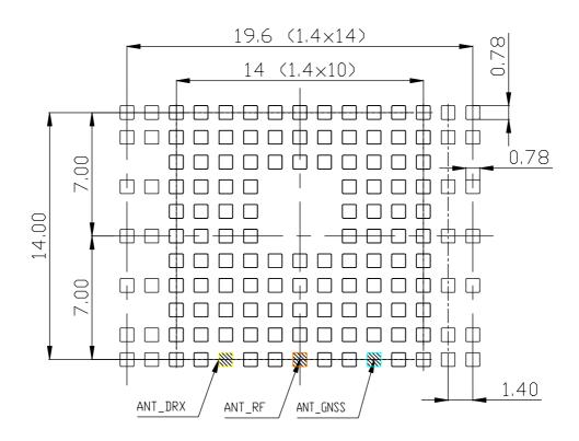
Figure 59: Land pattern TX82-W, TX62-W-B and TX62-W-C (top view)
