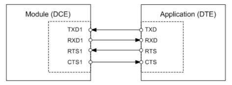
Figure 11: Serial interface ASC1
