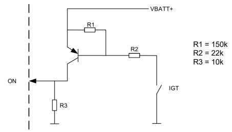
Figure 34: Sample ON circuit
