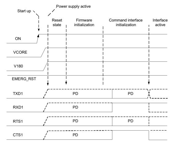
The following figure shows the startup behavior of the asynchronous serial interface ASC1.
