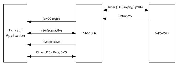
Figure 43: Handshake for module wake up after eDRX/PSM timer expiry
