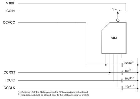
The figure below shows a circuit to connect an external SIM card holder.
