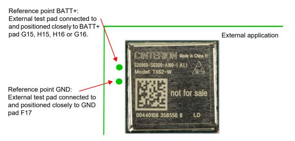
Figure 49: Position of reference points BATT+ and GND
