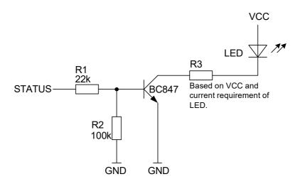
Figure 20: Status signaling with LED driver
