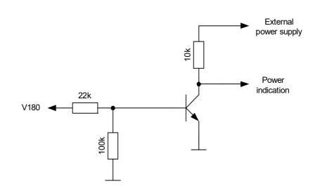
Figure 21: Power indication circuit
