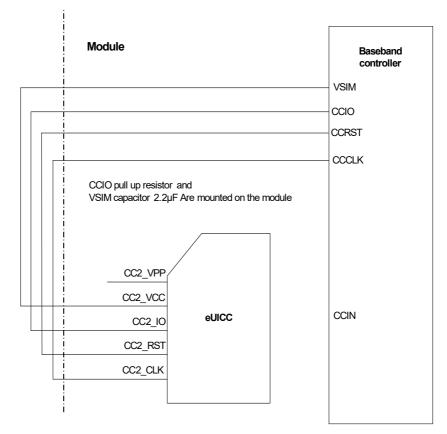
Figure 16: eUICC interface without SIM switch
