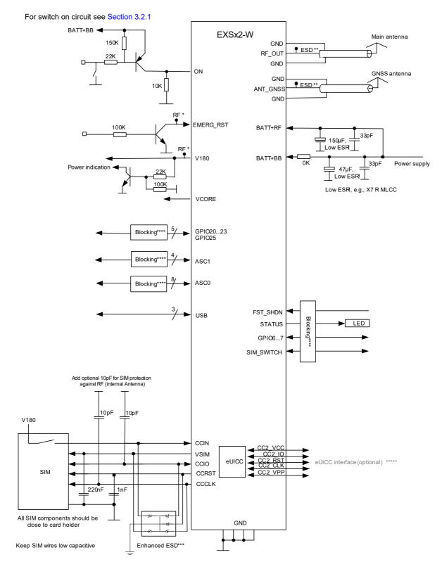
RF\* = Optional 47pF against self-interference. See also Section 3.6 for measures against RF interference ESD\*\* = ESD protection for RF antenna interface. For more details see Section 3.6.1 Enhanced ESD\*\*\* = Enhanced ESD protection for SIM interface. For more details see Section 2.1.6.1 Blocking\*\*\*\* = For more details see Section 3.6 eUICC interface\*\*\*\*\* = For more details see Section 2.1.7
