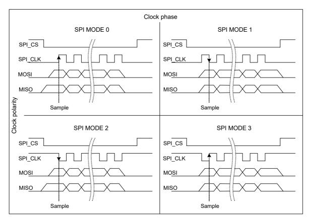
Figure 19: Characteristics of SPI modes
