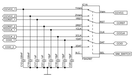
The SIM\_SWITCH signal is controlled by AT command (see [1]).
