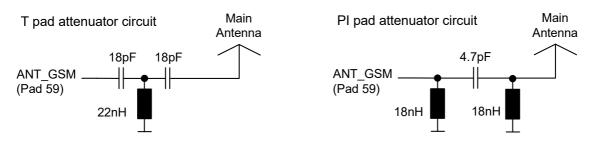
Figure 50: ESD protection for RF antenna interface
