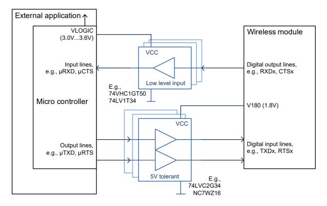
Figure 33: Sample level conversion circuit
