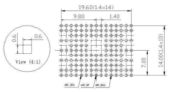
Figure 61: Recommended design for 110µm thick stencil for TX82-W, TX62-W-B and TX62-W-C (top view)
