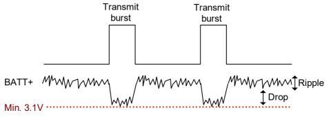
Figure 48: Power supply limits during transmit burst
