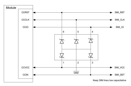
Figure 14: SIM interface - enhanced ESD protection
