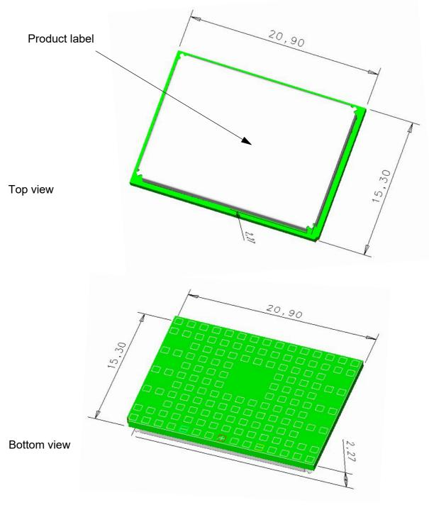
Figure 55: TX82-W- top and bottom view
