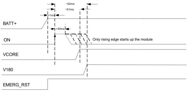
Figure 35: ON startup timing
