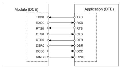
Figure 9: Serial interface ASC0
