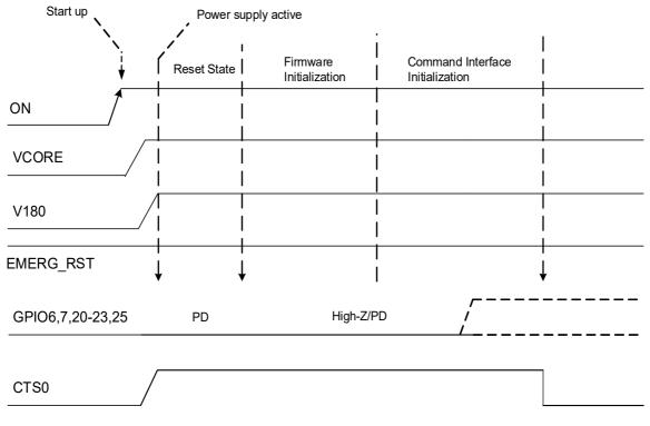
Figure 17: GPIO start up behavior
