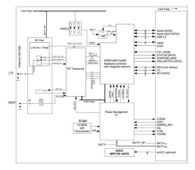
Figure 4: TX62-W-B block diagram
