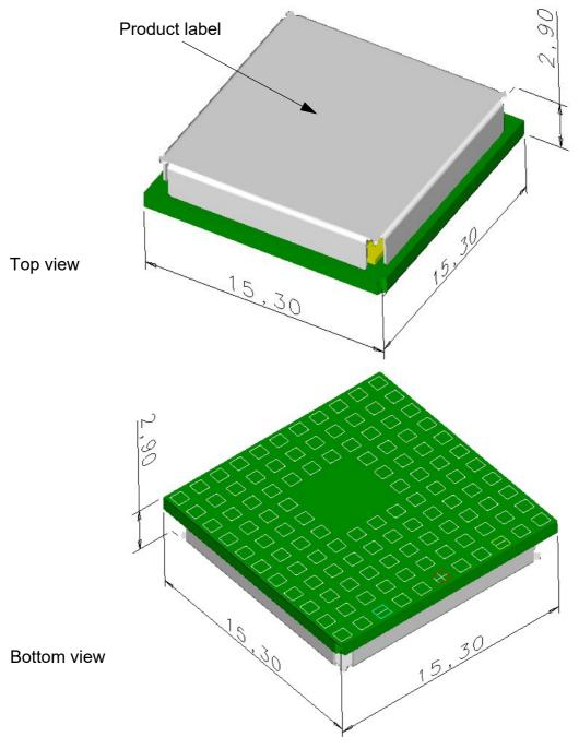
Figure 52: TX62-W- top and bottom view
