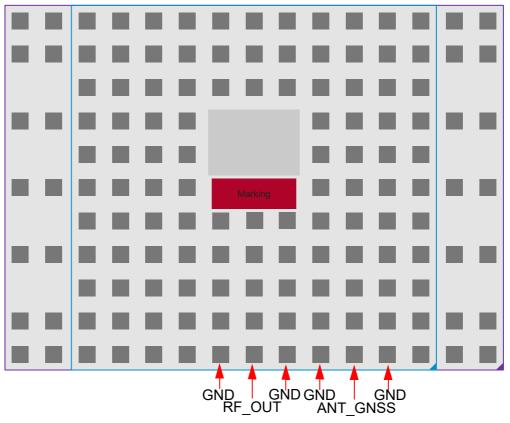
Figure 24: Antenna pads (top view)
