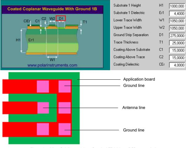
Figure 27: Micro-Stripline on 1.0mm Standard FR4 2-layer PCB - example 2
