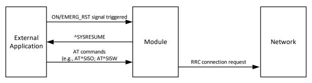
Figure 42: Handshake for module wake up via ON signal
