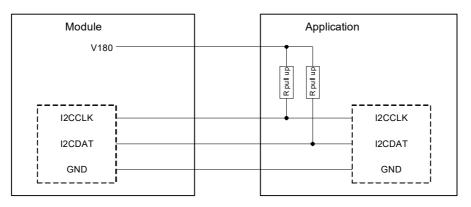
**Figure 18:** I<sup>2</sup>C interface connected to V180
