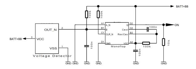
Figure 36: Automatic switch ON circuit sample
