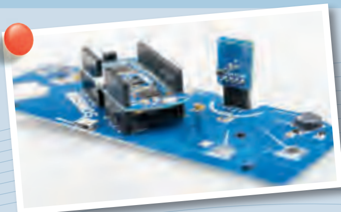
◀ Board with temperature sensor
