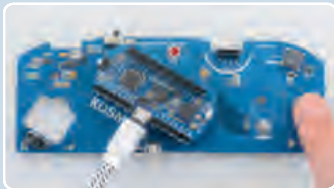
▲ Finger pushes right button — NeoPixel glows red
