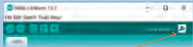
▲ A click on the magnifying glass at the upper right will launch the serial monitor.
