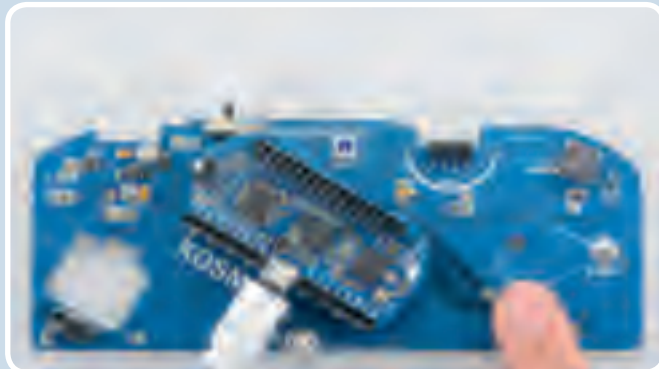
▲ Finger pushes left button — NeoPixel glows blue
