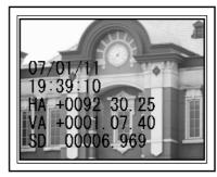
Survey data recorded during taking pictures can be displayed on the screen. The image data taken during special function such as measure can be recorded on coordinated data in addition to Polar data and these data can be displayed in due course.
