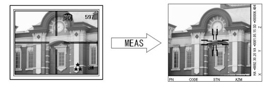
Aim the target when using the telescope or the camera display. Press [F3] [SNAP] key to take a shot.
