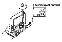
**Step 4.** Adjust the corresponding tuner's volume control so that its knob points to the 2 o'clock position. If the tuner's AF PEAK indicator remains lit, readjust the microphone's audio level control to the position that causes the indicator to flash when the tuner output level reaches its peak. The AF PEAK indicator lights when the output level reaches the point of about 3 dB below the clipping level.
