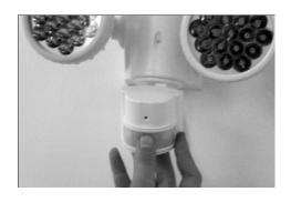
7) Adjust the motion detection sensor and cameral towards the desired coverage area.
