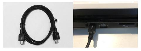
2. Plug the other end of the special USB cable with marked "MDT" to the Device or the Cradle
