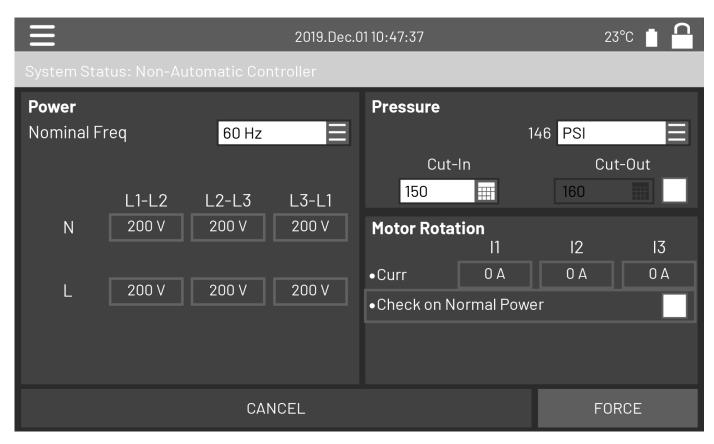
Once the controller has booted up, the "First Start Up" page appears. The controller will automatically detect and display the frequency of the power source. It is then possible to manually choose the frequency of the voltage.
