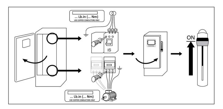
Make sure to drill holes for the motor and power connections and run the cables inside the panel, all in accordance with the specifications in order to minimize interference with other equipment.
