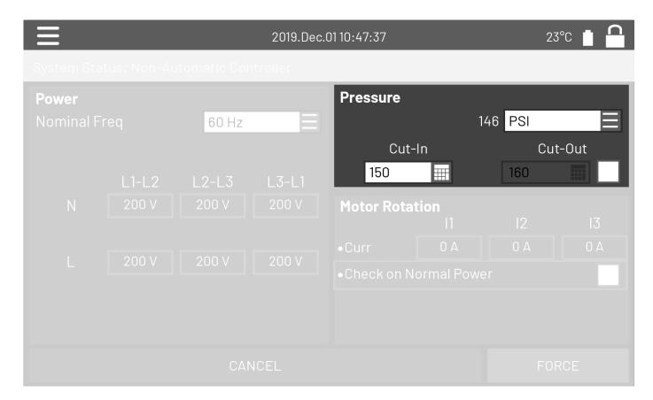
Choose the desired units of measurement for pressure reading and verify that it matches with the calibrated pressure gauge installed on the sensing line. Set the Cut-In value according to your system specifications. Cut-Out value will default to Cut-In plus 10 PSI. To manually enter the cut-out, select the check-box besides it and enter the desired value (optional).
