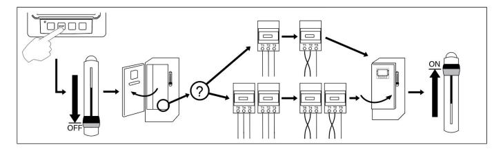
Connect the input power and the motor on their respective terminals. Secure with the appropriate torque as indicated on the torque label and verify all connections. Secure the door in closed position then put the circuit breaker disconnecting means in ON position. Verify the readings on the controller main screen.
