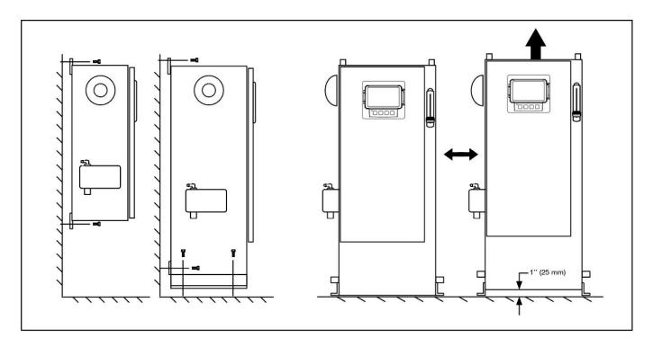
Verify that the controller is installed securely on the wall, or optionally on the mounting stand.
