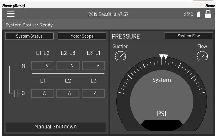
The home page displays all controller statuses and important values of the controller. This includes all voltages, currents, pressures, motor state and status
