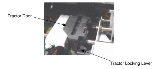
Raise the tractor doors and fit the first two paper feed holes onto the right tractor pins.
