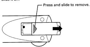
Place two "AA" size alkaline batteries, matching the + and - signs on each battery to the + and - signs of the battery compartment.
