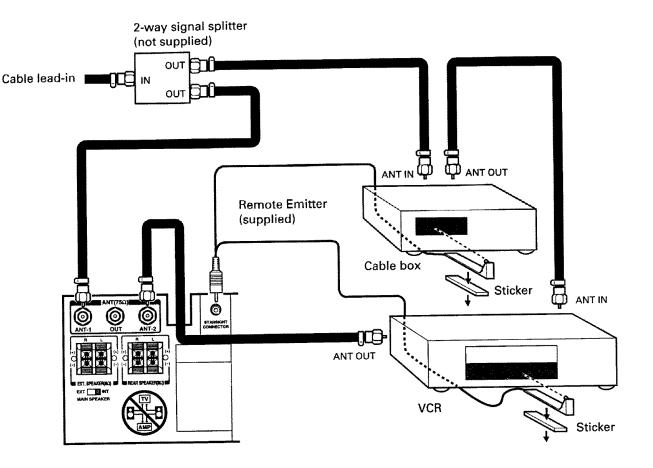
The unscrambled channels will come through the ANT-1 terminal whenever the antenna input is set to "ANT 1" mode. The scrambled channels, after decoded by the cable box, will come through the VCR and the ANT-2 terminal whenever the antenna input is set to "ANT 2" mode (see page 36). Select channel 3 or 4 on your TV and VCR to match your cable box's output channel.
