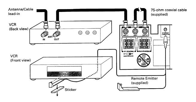
Note: On many VCR's, playing tapes causes the VCR's TV/VCR switching to disconnect the antenna signals from the TV. If you cannot select a certain channel, try pressing the TV/VCR button on the Remote Control.
