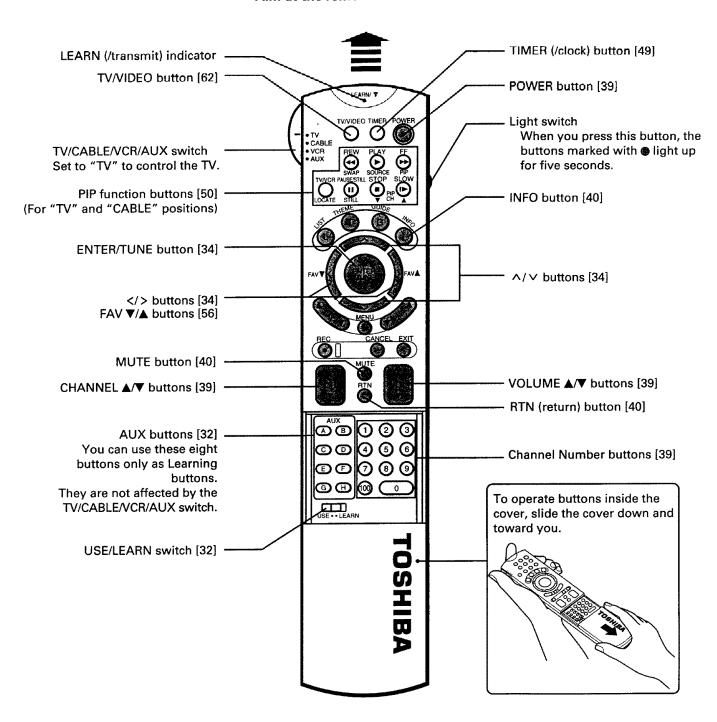
Note: The TV/VIDEO, TIMER, PIP, INFO, ^/∨/</>, ENTER/TUNE, MENU, EXIT, MUTE and VOL ▲ / ▼ buttons will always operate this TV regardless of the TV/CABLE/VCR/AUX switch setting.
