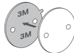
2. Stick the mental plate with adhesive to a clean wall. Then attach the camera to the plate.
