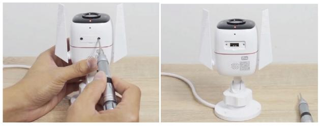
2. Identify the direction of the microSD card and carefully insert the card into the slot. Push in the card until you hear a clicking sound.
