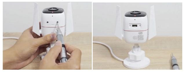
2. Press and hold the Reset button for at least 5 seconds until the LED blinks red.
