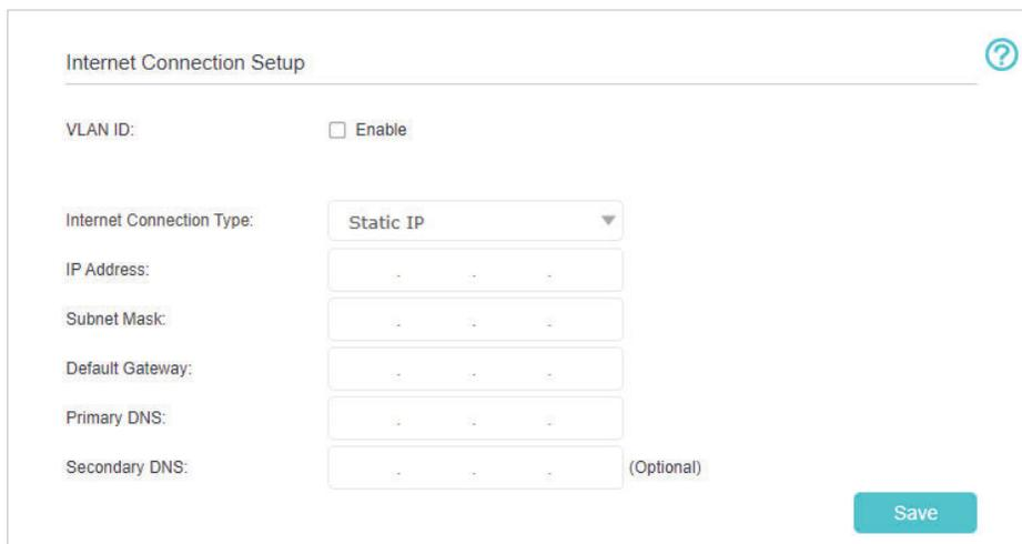
The screenshot shows the 'Internet Connection Setup' page. At the top, there is a title 'Internet Connection Setup' with a help icon. Below it, there is a 'VLAN ID' section with an 'Enable' checkbox. Underneath, the 'Internet Connection Type' is set to 'Static IP' in a dropdown menu. Below this, there are input fields for 'IP Address', 'Subnet Mask', 'Default Gateway', 'Primary DNS', and 'Secondary DNS' (marked as optional). A 'Save' button is located at the bottom right of the form.
