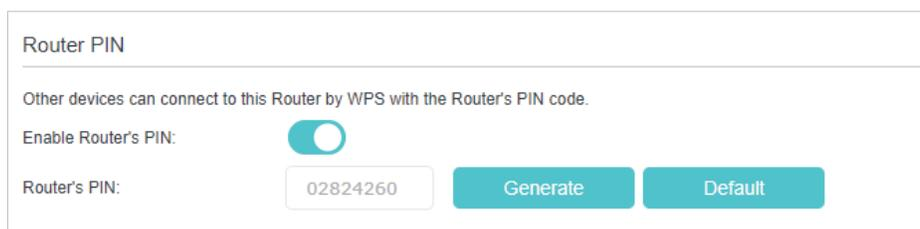
3. Take a note of the current PIN of the router. You can also click the [Generate](#) button to get a new PIN.
