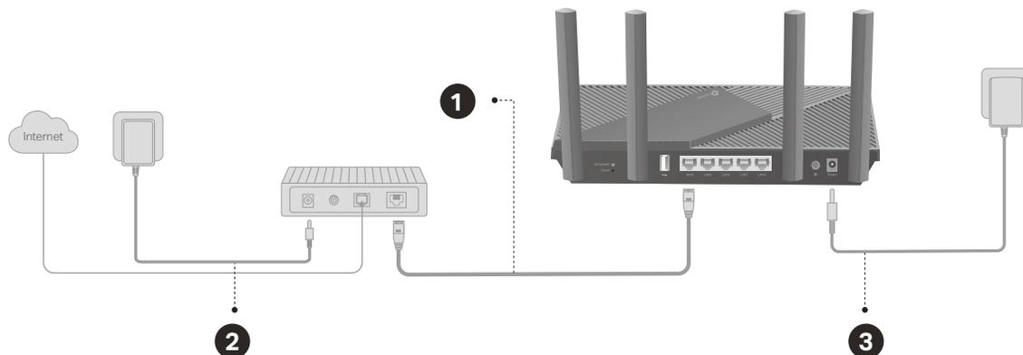
1. Connect the modem to the router's WAN port with an Ethernet cable.
