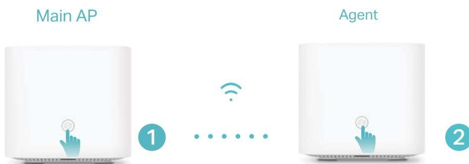
3. The status LED will flash blue fast for about two minutes during the synchronizing process.
