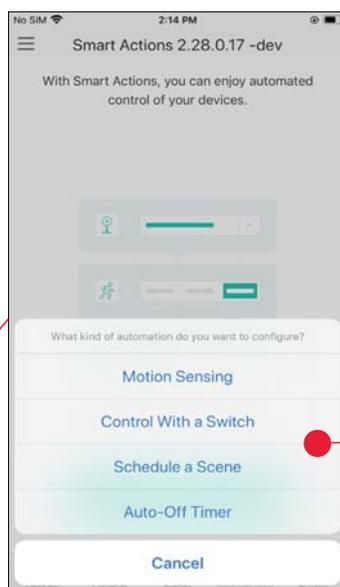
**Motion Sensing:** Take actions when a Kasa camera senses a motion.
