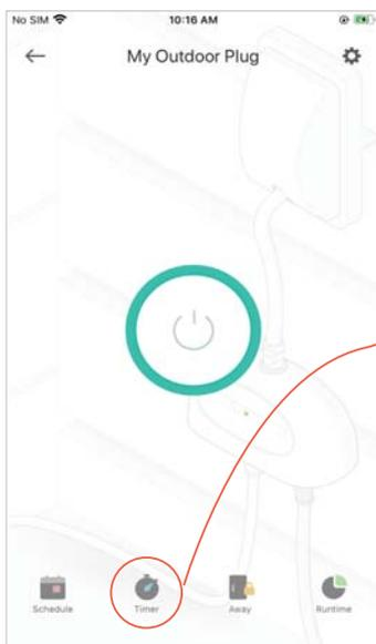
2. Set the time after which the plug will be automatically turned on/off.
