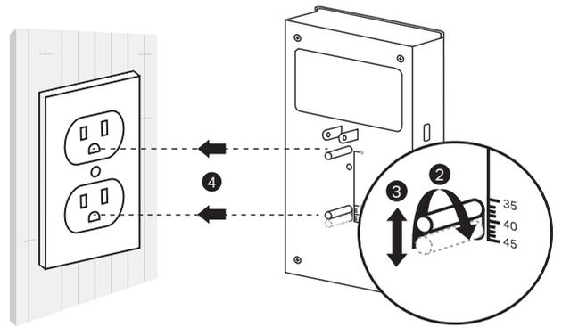
**Note:** The removable stabilizing post makes the device fit any type of wall socket, such as a duplex outlet, decorator outlet, USB receptacle, or GFCI outlet.
