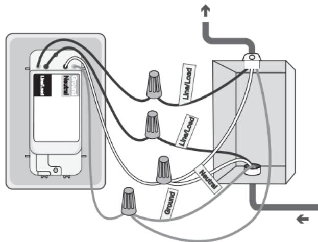
Note: No need to distinguish between Line and Load wires.
