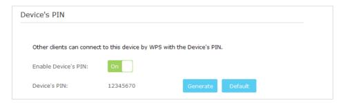
1) Toggle On Enable Device's PIN to allow wireless clients to connect to the device using the Device's PIN.
