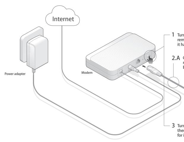
Turn off the modem and remove the backup battery if it has one.
