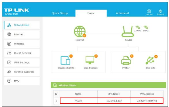
3. On a computer that connects to the same router as the camera does, open a web browser, type in the camera's IP address in the address field, and press **Enter**. Here we use http://192.168.1.103 for demonstration.
