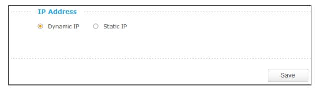
> Static IP: Select this option when a static or fixed IP address is obtained for the camera. A static IP address will ease your access to the camera in the future. Add your camera's static IP information to your router to avoid IP conflicts.
