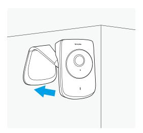
After relocating your camera, face it towards the area you'd like to view, and then plug the power adapter into a power outlet.
