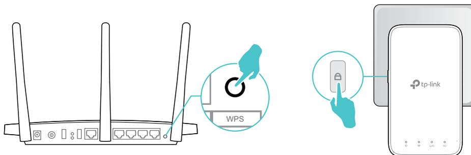
2. Wait until the Signal LED
