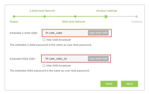
5) Verify your wireless settings and click **Finish**. The corresponding LEDs (2.4GHz and 5GHz) should turn on and stay solid.
