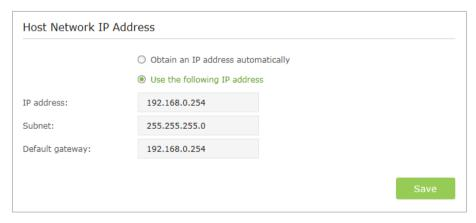
IP Address: Enter the IP address in dotted-decimal notation (192.168.0.254 by default).
