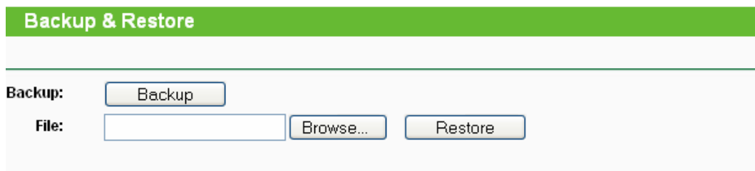
Figure 4-38 Save or Restore the Configuration
