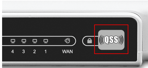
Figure 3-15 Press the QSS Button
