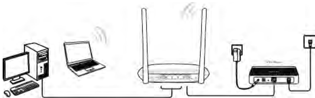
Figure 2-2 Hardware Installation of the TL-WR843N in Router mode
