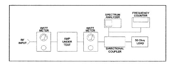
TEST SET UP FIGURE 1
