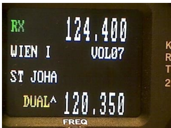
Figure 4: KRT2 active & standby frequencies
