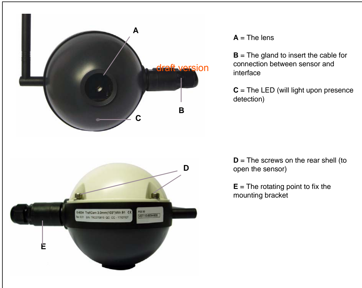
Figure 4: Front and side view of the TrafiCam® sensor
