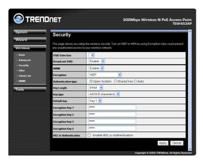
**ESSID Selection:** As this device supports multiple SSIDs, it is possible to configure a different security mode for each SSID (profile). Select an SSID from the drop-down list.
