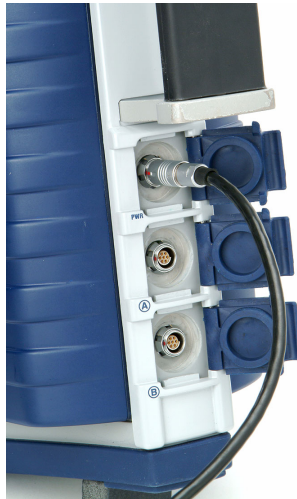
Figure 3 Connecting External Power to Main Module
