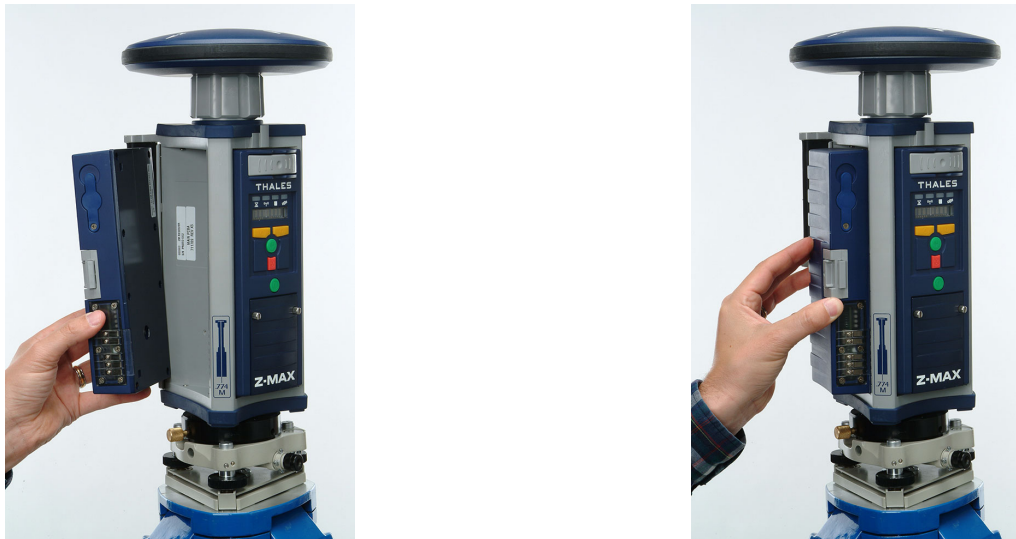
Figure 2 Power Module and GPS Receiver Module
