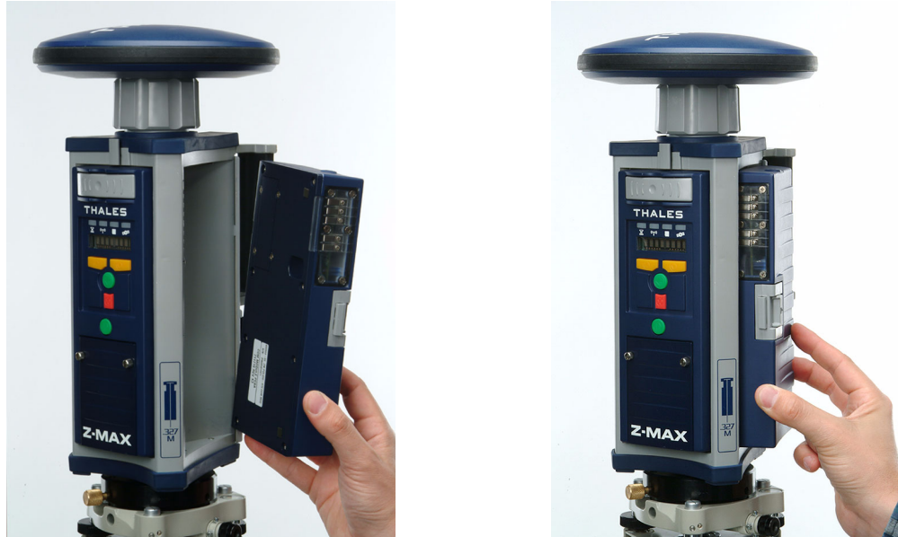
Figure 5 Connecting Communication Module
