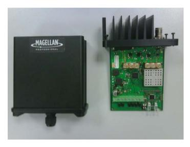
The U-Link TRx must be supplied from a DC voltage source. The input DC power voltage range is 9V up to 28V, and the total power consumption is less than 1.5A under 12V at full RF power with an antenna connected on the RF port output.
