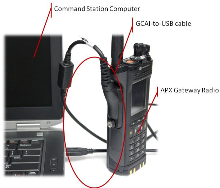
Figure 252. Motorola APX Radio connected to a Command Station using a GCAI cable.
