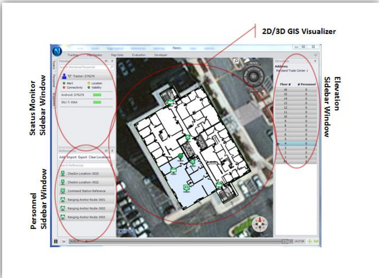
Figure 3. Neon Tracking with sidebar windows expanded to monitor tracking.
