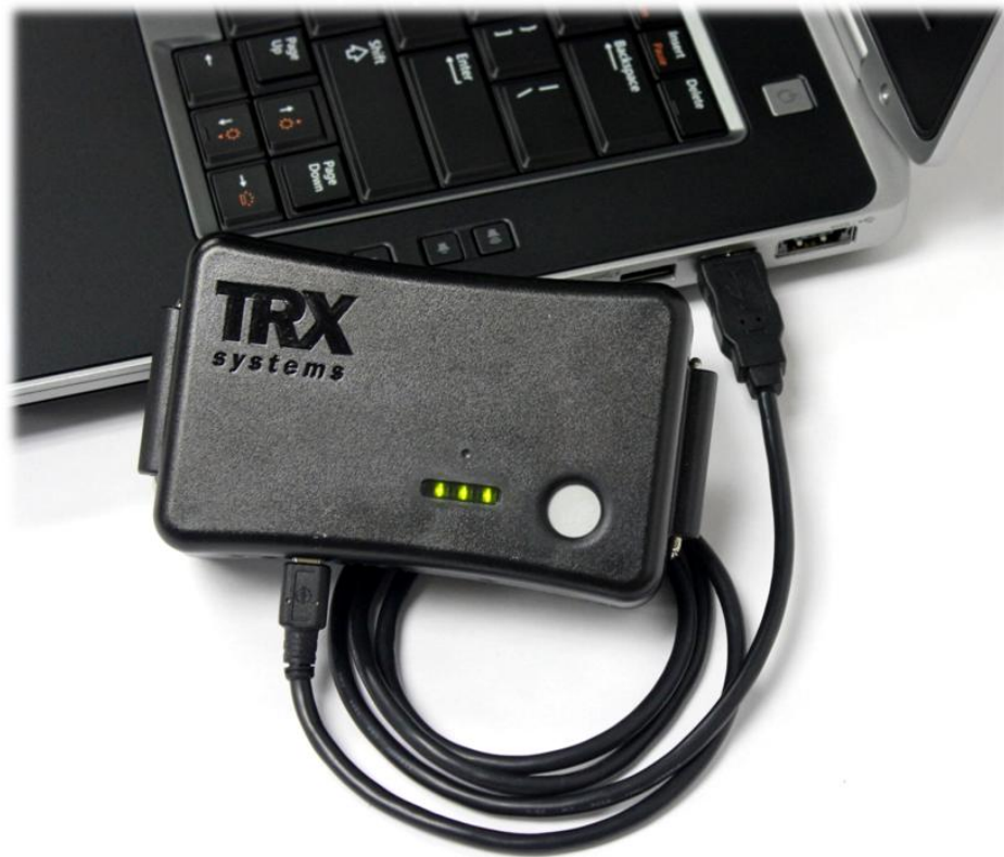
Figure 44. The Command Software Reference is attached directly to the computer hosting the Neon Command Software.
