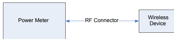
Figure 5-1 Power Measurement Setup
