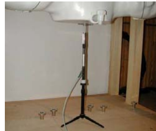
Figure 6-2 System Verification Setup Photo
