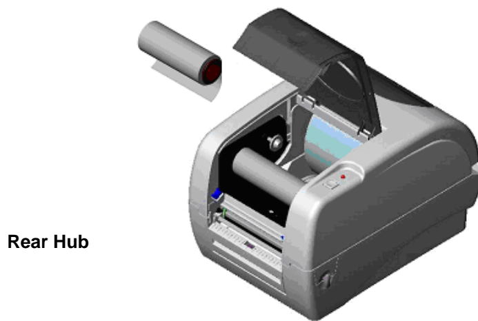
Fig. 5 Ribbon installation (II)
