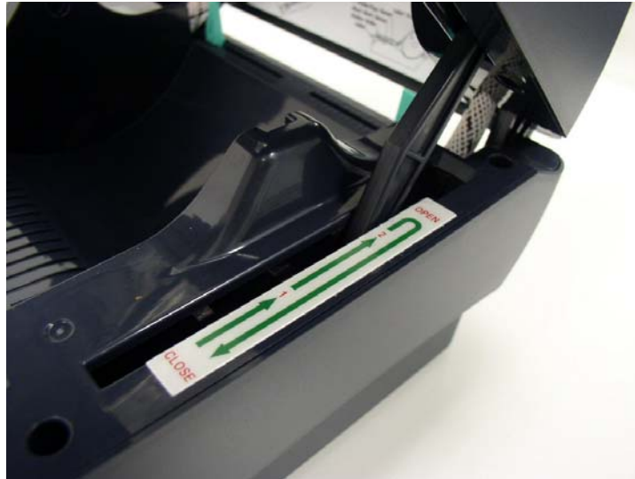
Fig. 1 Top cover support is fixed at position 2
