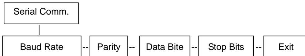
For desktop printer models, the RS-232 communication parameters can be setup following command
