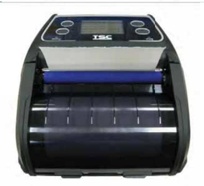
4. Press each side of media cover to close the media cover and make sure the media cover closed correctly.
