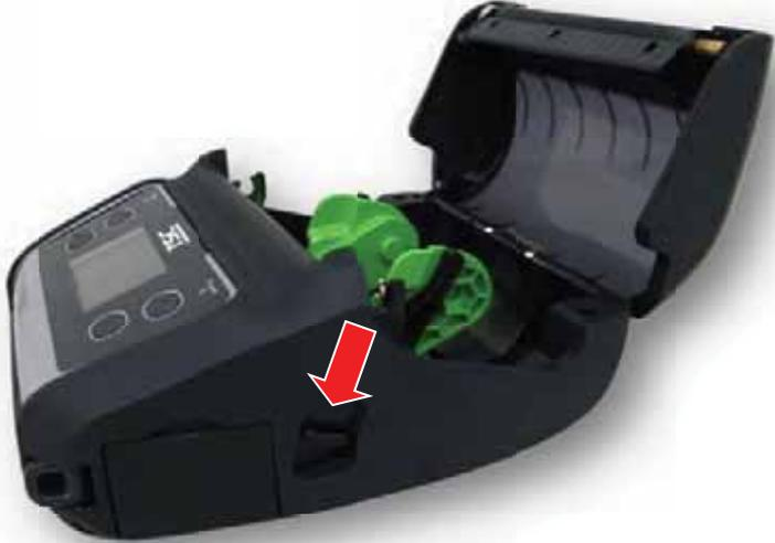
A photograph of a black TEC printer with its media cover open. A red arrow points to a small button on the front of the printer, which is the media cover release button.                           | <p>1. Open the printer media cover by pressing the media cover release button.</p>
