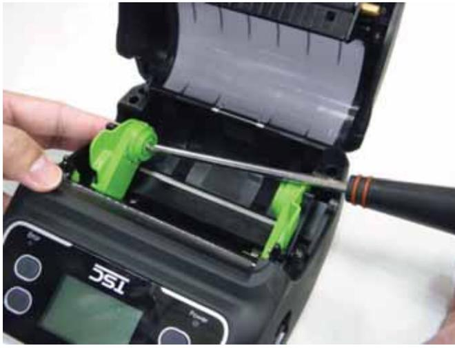
5. Tighten the screw on nut for fixing the adapter on media holder.
