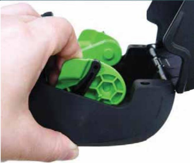
1. Open the printer media cover by pressing the media cover release button. Pull the media holders apart to fit the media width.
