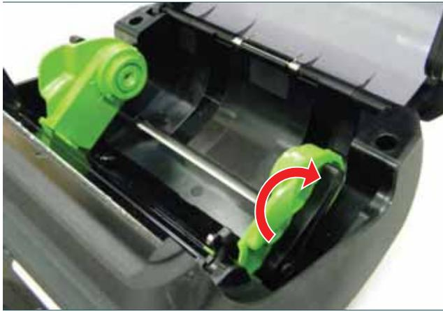
4. Pull the media holders apart. Push down another side of media holder lock switch to keep the media holder in max width.
