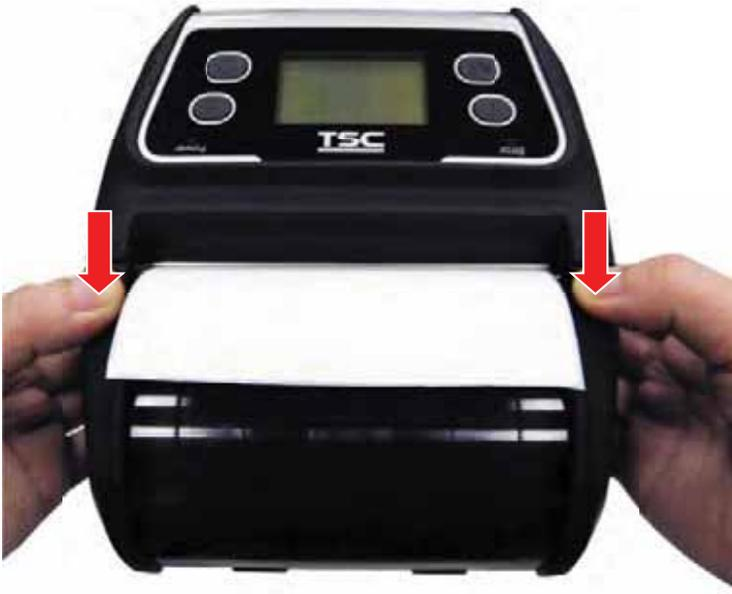
4. Press each side of media cover to close the media cover and make sure the media cover closed correctly.
