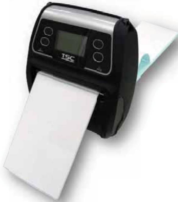
4. Press each side of media cover to close the media cover and make sure the media cover closed correctly.
