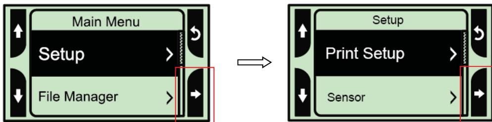
2. Press button to enter the “Print Setup” item. Select the “TSPL2” item. Enter the “Speed” setting mode.
