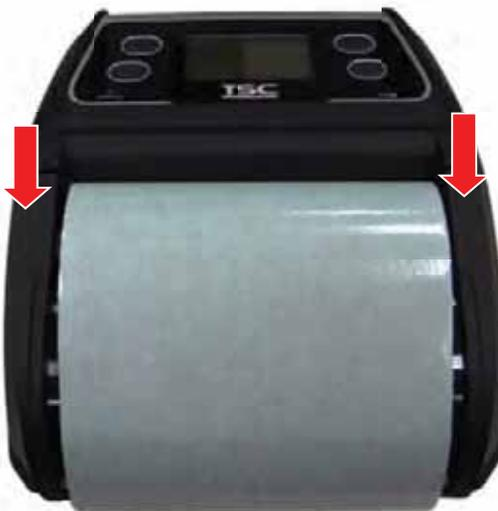
3. Press each side of media cover to close the media cover and make sure the media cover closed correctly.
