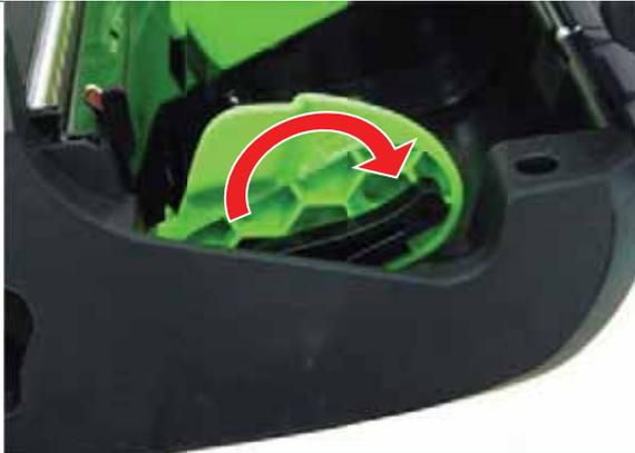
2. Push down each side of media holder lock switch to fix the media holder.
