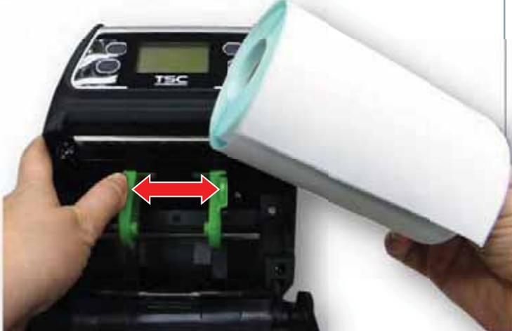
A photograph showing a person's hands pulling two green media holders apart. A red double-headed arrow indicates the direction of movement. A roll of white paper is being held above the holders. | <p>2. Pull the media holders apart to fit the label roll width.</p>
