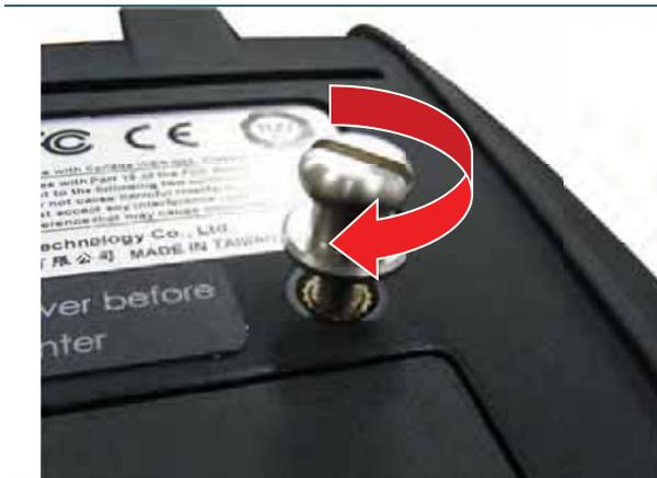
1. Tighten 2 screws on the printer.
