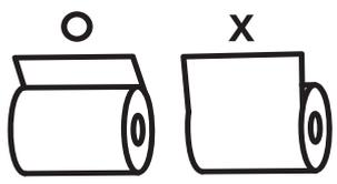
A diagram enclosed in a dashed box. It shows two side views of a roll of paper. The left view shows the roll with a small circle on top, representing the correct loading method. The right view shows the roll with an 'X' on top, representing an incorrect loading method.</div> |
