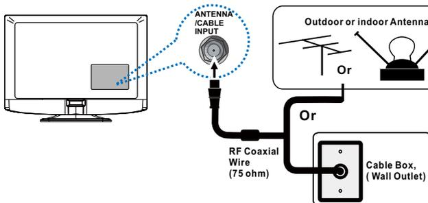
Connect the RF coaxial cable on your home outlet to the **ANTENNA/CABLE INPUT** jack of this unit.
