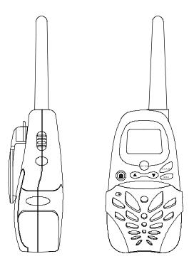
1) PTT switch : Push and hold to transmit ; release to receive.
