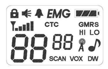
Key lock indicator: Indicates that the key lock function is in use
