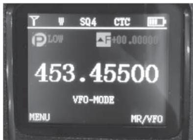
The radio work in the analog mode, and you only can transmit and receive in the analog mode, and whatever you press which PTT key, it will transmit in the analog mode.
