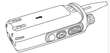
2. To move the battery, please make sure the radio is closed, push the battery latch up, and then push the battery out from the radio.
